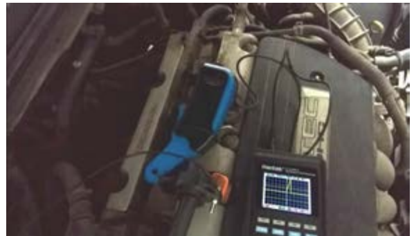
Primary ignition current test
