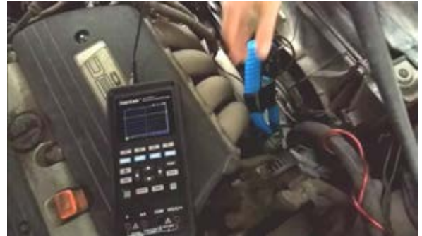
Charging circuit current and voltage test
