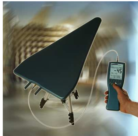
Spectrum Analyser and HyperLOG® directional antenna
